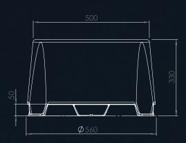
Made from recycled cast iron, top diameter of 56cm/22", height 33cm/13" Weight of the product up to 43kg/117 pounds
